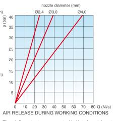
The air flow charts were created in Kg/s from laboratory tests and numerical analysis, without the screen, then converted in Nm³/h using a safety factor.
