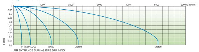
The air flow charts were created in Kg/s from laboratory tests and numerical analysis without the screen, then converted in Nm<sup>3</sup>/h using a safety factor.
