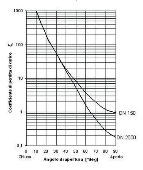
Determinates the head loss  $\Delta h$  it's possible to calculate the flow rate Q in m3/h with the following expression (the same expression can be used to, having the project flow rate Q, to determinate the head loss  $\Delta h$  without using the head loss coefficient):
